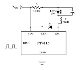
A value of 1uF will reduce the supply ripple current by a factor three (approx.). Proportionally lower ripple can be achieved with higher capacitor values. Note that the capacitor will not affect operating frequency or efficiency, but it will increase start-up delay and reduce the frequency of dimming, by reducing the rate of rise of LED voltage.
