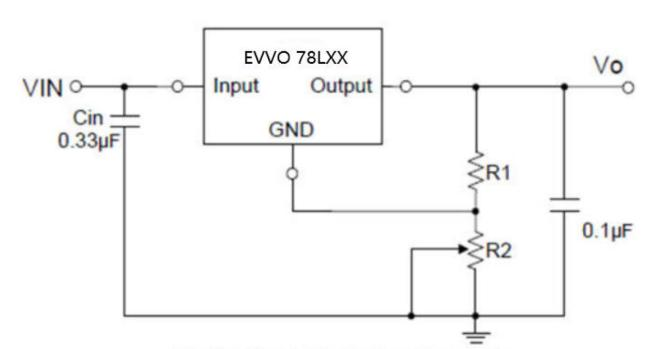
Fig.3 Adjustable Output Regulator
